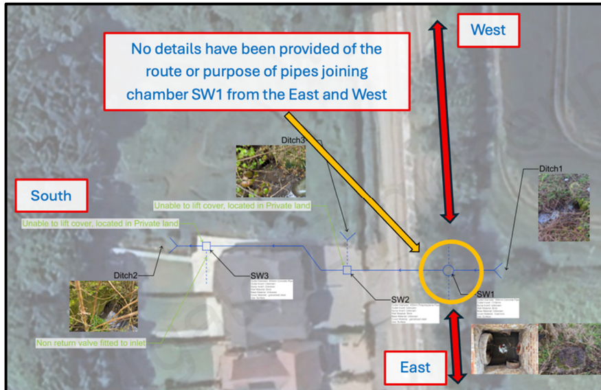
Fig 1 Directional run of pipes that join inspection chamber SW1 from the East and West.
